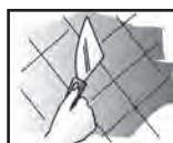
Gently score the areas to be stripped using a proprietary perforator tool or the edge of a wall scraper in a criss-cross pattern.
